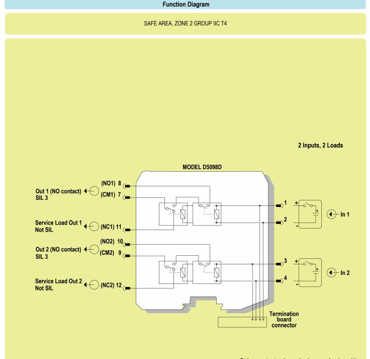
Relay contacts shown in de-energized position. Terminals 7-8 and 9-10 are open; terminals 7-11 and 9-12 are closed.
