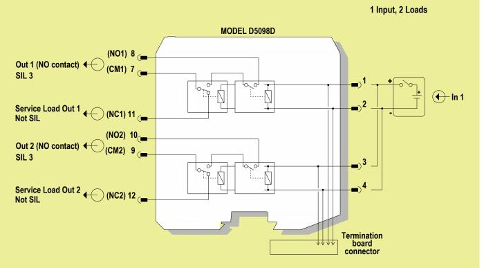
Relay contacts shown in de-energized position. Terminals 7-8 and 9-10 are open; terminals 7-11 and 9-12 are closed.
