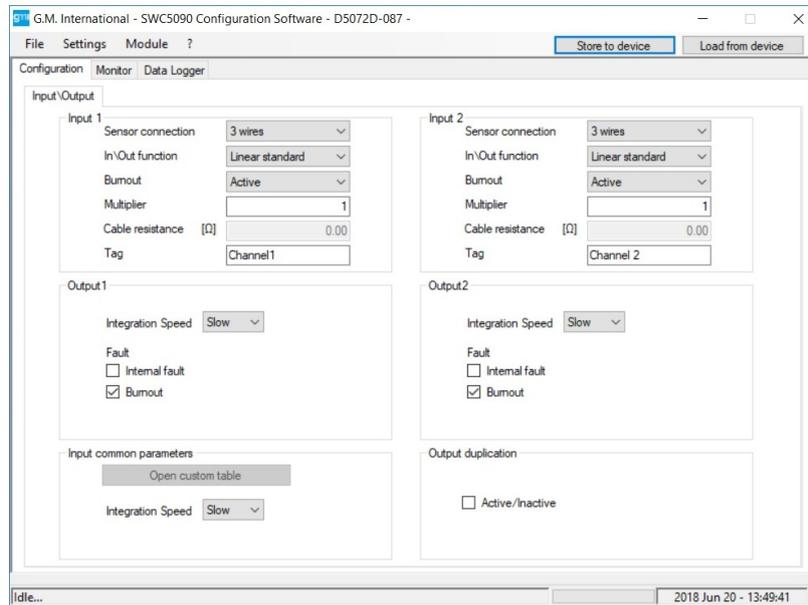
**Figure 19: D5072D-087 Input / Output configuration screen.**
