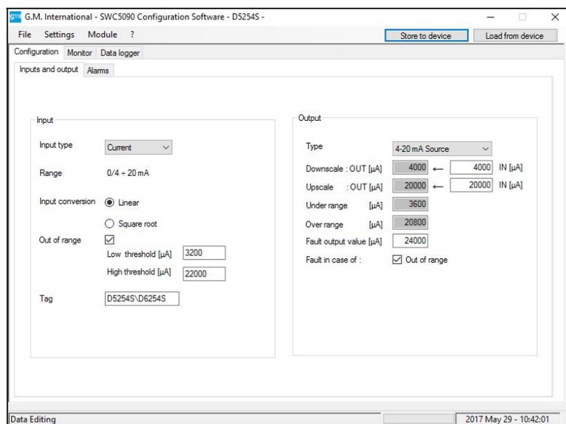
**Figure 59: D5254S / D6254S Input / output configuration screen.**
