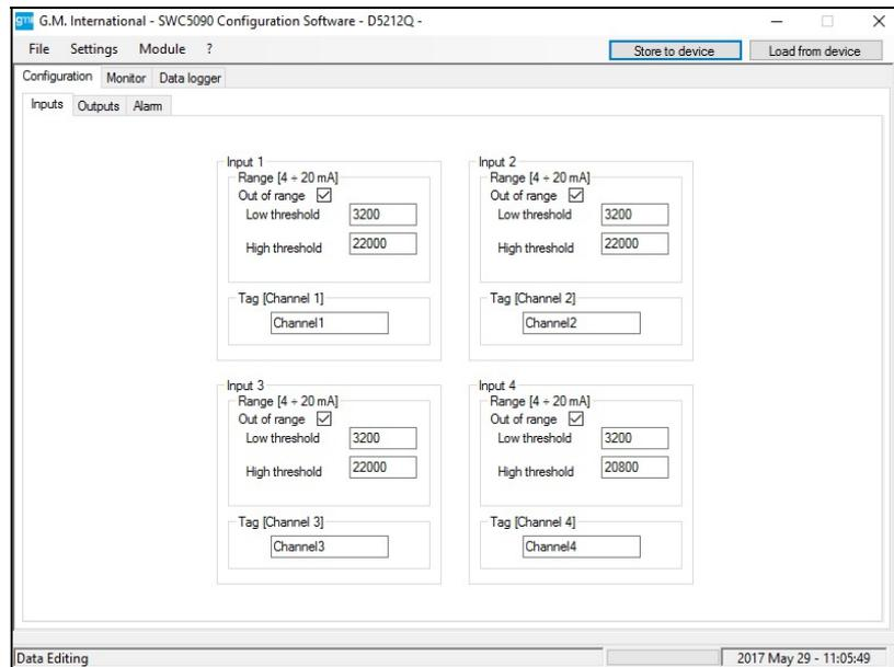
**Figure 63: D5212Q / D6212Q Input / output configuration screen.**
