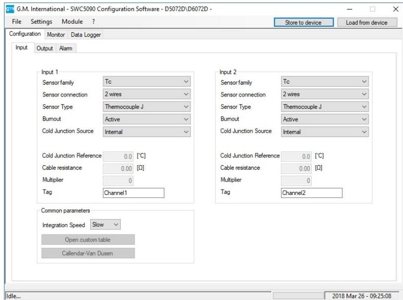
**Figure 14: D5072D / D6072D Input configuration screen.**
