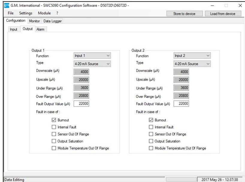
**Figure 10: D5072D / D6072D Output configuration screen.**
