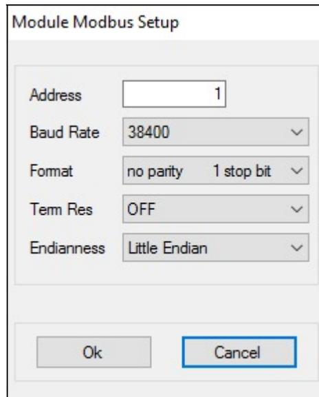
**Figure 6: Modbus Setup window.**
