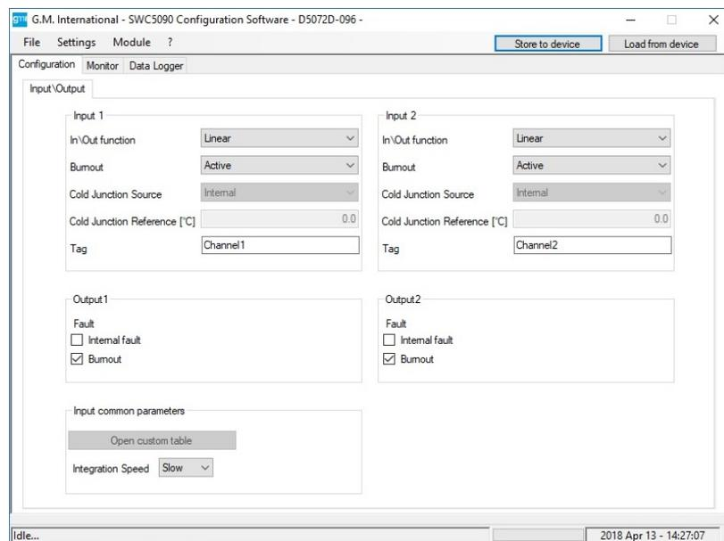
**Figure 22: D5072D-096 Input / Output configuration screen.**
