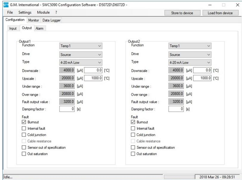
**Figure 15: D5072D / D6072D Output configuration screen.**
