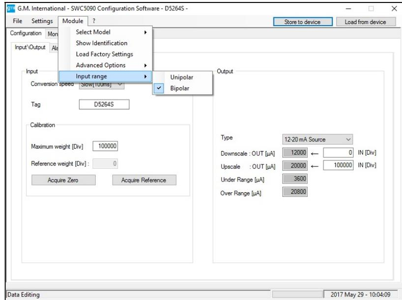
**Figure 55: D5264S Input / output configuration screen.**
