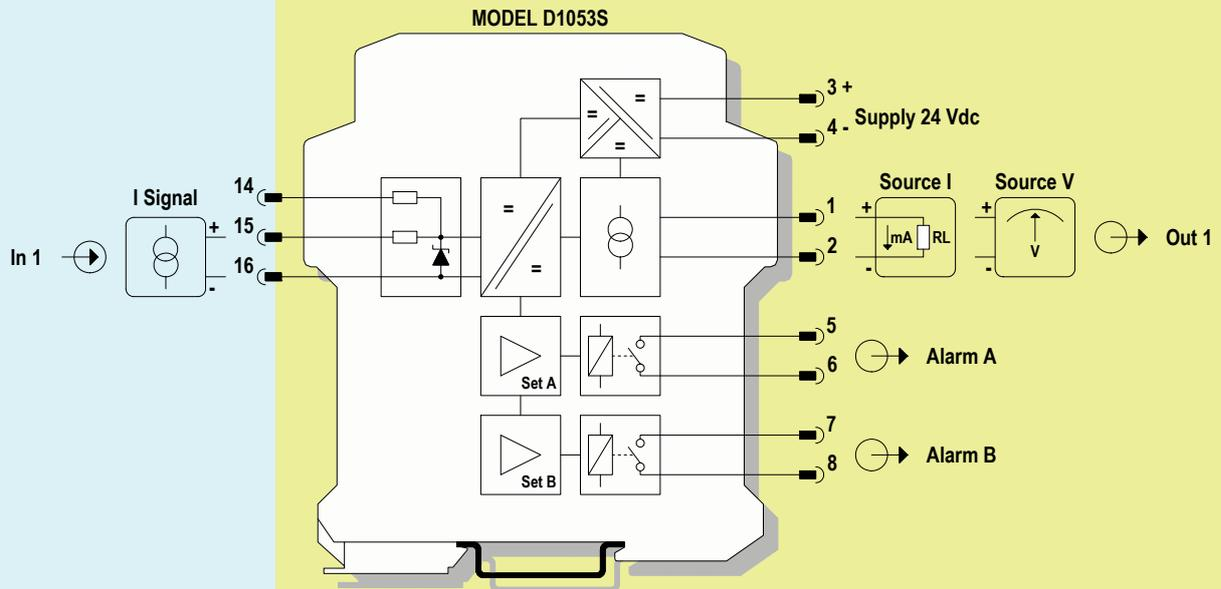
For SIL applications, alarm contacts must be used in series with equal configuration. Relay contact shown in de-energized position
