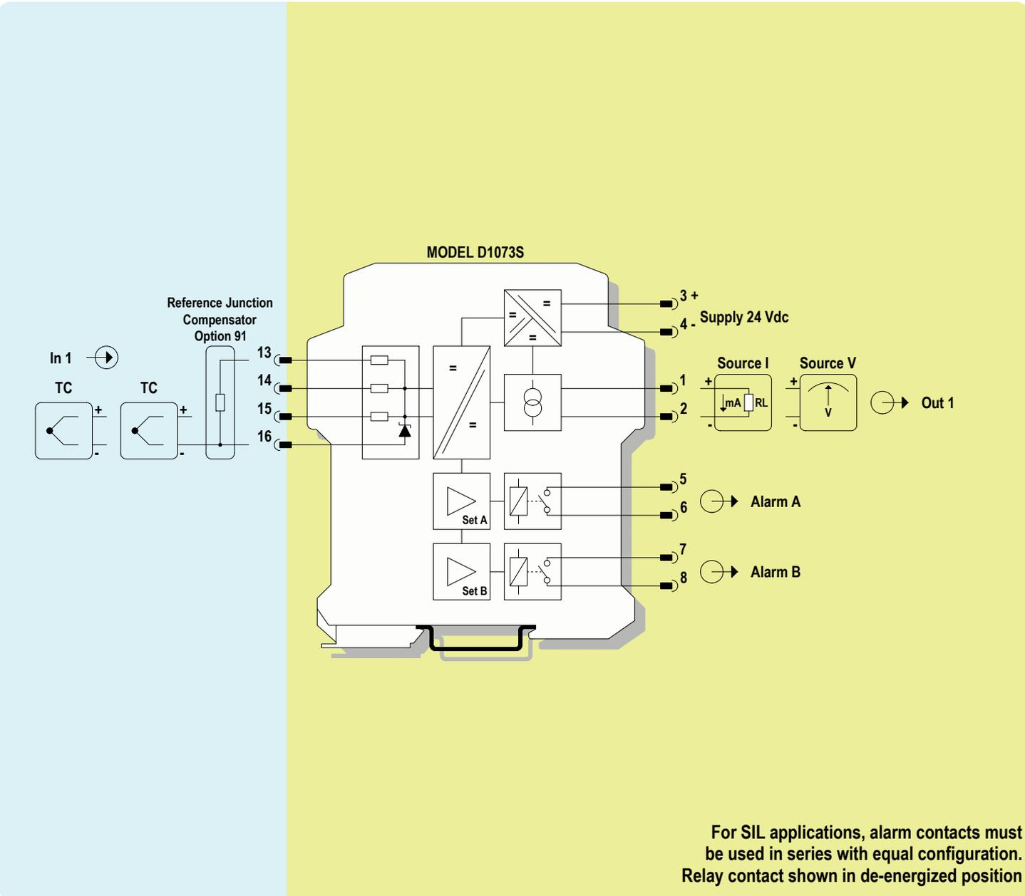
For SIL applications, alarm contacts must be used in series with equal configuration. Relay contact shown in de-energized position
