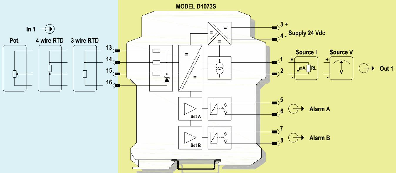
**For SIL applications, alarm contacts must be used in series with equal configuration. Relay contact shown in de-energized position**
