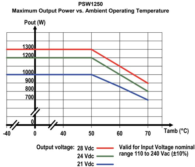
With 50% redundant configuration (two PSW1250 with paralleled outputs), each module can give 600 W power output up to 70°C operating ambient temperature, with output voltage range 21-28 Vdc and input voltage nominal range 110+240 Vac ( $\pm 10\%$ ).
