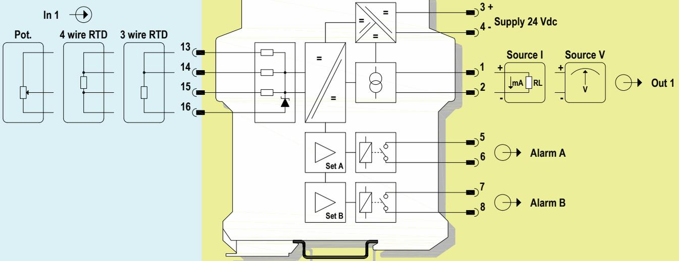
**For SIL applications, alarm contacts must be used in series with equal configuration. Relay contact shown in de-energized position**
