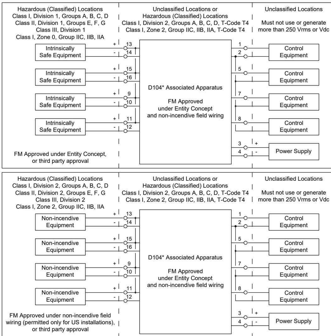
**NOTE: outputs can be paralleled to increase output power. When combining outputs, consider Safety Parameters matching with the field device and allowable Group as shown in the Safety Parameters Table and check that requirements are met.**
