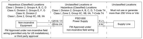
Non-incendive field wiring is not recognized by the Canadian Electrical Code, installation is permitted in the US only.
