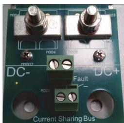
PSW1250 screw output terminals on copper bars:
