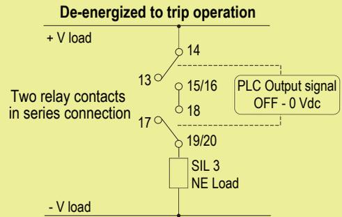
SIL 3 Normally Energized Relay Condition for ND Load
