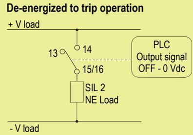
SIL 2 Normally Energized Relay Condition for ND Load
