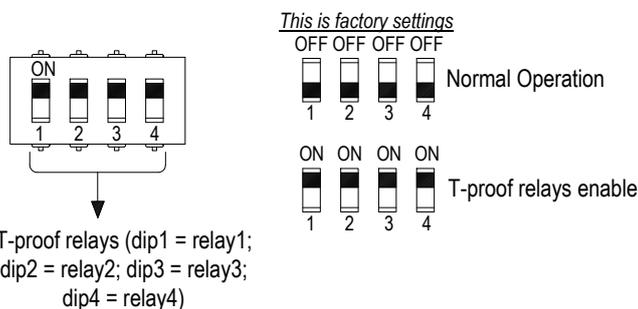
**WARNING: after T-proof test, dip-switch 1-2-3-4 must be set to "OFF" position for normal operation.**
