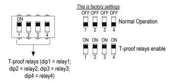
WARNING: after T-proof test, dip-switch 1-2-3-4 <u>must be</u> set to "OFF" position for normal operation.
