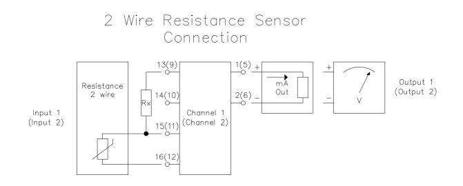
Rx Value: must be equal to maximum value of resistance to obtain 50% full scale value (input connection as for 3 wire transmitting potentiometer).
