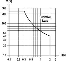
DC Load breaking capacity:
