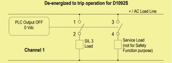
Contacts 1-2: the SIL 3 Safety Function is met when the relay is de-energized, contact is open, SIL 3 load is de-energized.
