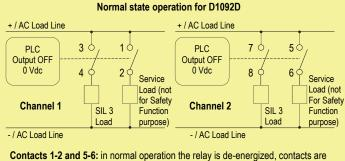
open, Service Load loads (not for Safety Function purpose) are de-energized
