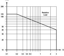
Mechanical / Electrical life: 50 \* 106 / 1 \* 105 operation, typical. Operate / Release time: 5 / 3 ms typical.
