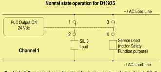
Contacts 1-2: in normal operation the relay is energized, contact is closed, SIL 3 load is energized.
