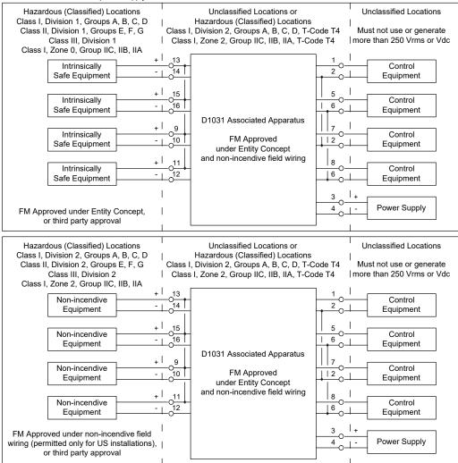
Non-incendive field wiring is not recognized by the Canadian Electrical Code, installation is permitted in the US only.
