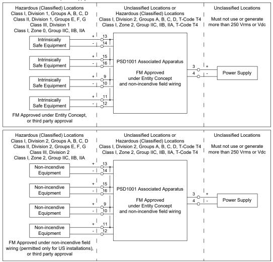
NOTE: outputs can be paralleled to increase output power. When combining outputs, consider Safety Parameters matching with the field device and allowable Group as shown in the Safety Parameters Table and check that requirements are met.
