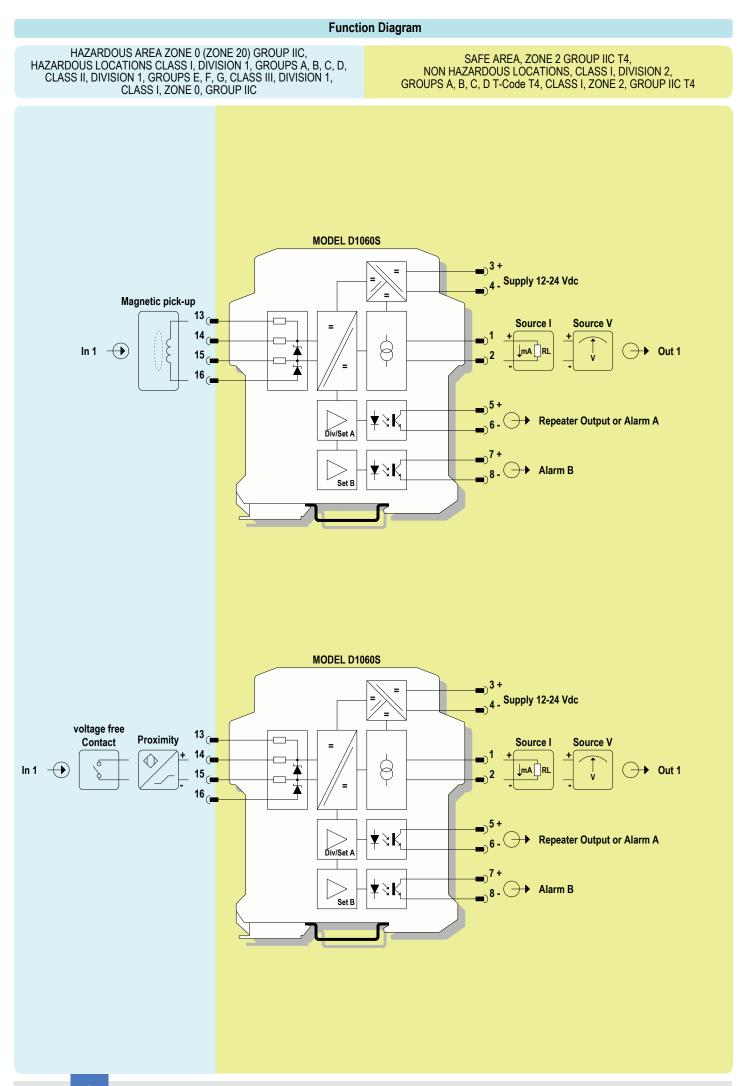
D1060 - Frequency - Pulse Converter, Repeater and Trip Amplifiers
