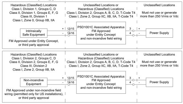
Non-incendive field wiring is not recognized by the Canadian Electrical Code, installation is permitted in the US only.
