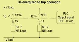
SIL 2 Normally Energized Relay Condition for ND Load
