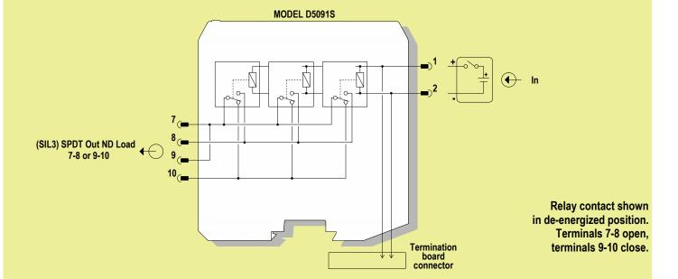
SIL3 Safety Function for ND load (energized in fail safe state) is available at terminal blocks 7-8; In this case, the Safety Function is met when the relay is energized (closed contact).
