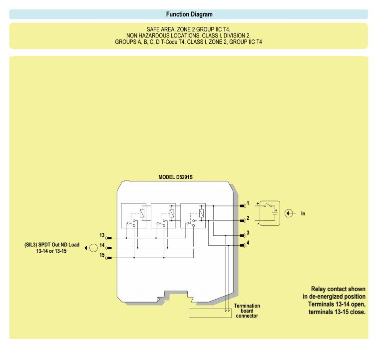
SIL3 Safety Function for ND load (energized in fail safe state) is available at terminal blocks 13-14; In this case, the Safety Function is met when the relay is energized (closed contact).
