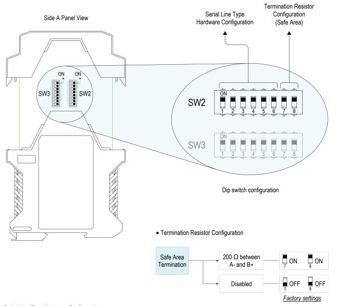
• Serial Line Type Hardware Configuration
