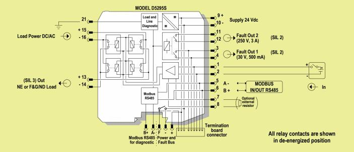
To prevent relay contacts from damaging, connect an external protection (fuse or similar), chosen according to the relay breaking capacity diagram.
