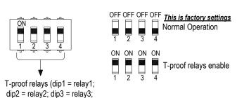
WARNING: after T-proof test, dip-switch 1-2-3-4 <u>must be</u> set to "OFF" position for normal operation.
