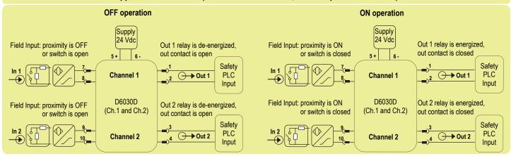
**Description:** For this application, enable input line fault (open or short) detection and direct input to output transfer function, by set the internal dip-switches in the following mode (see pages 7 and 8 for more information):
