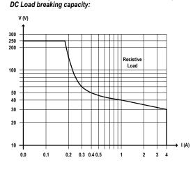
Mechanical / Electrical life: 5 \* 106 / 3 \* 104 operation, typical. Operate / Release time: 8 / 4 ms typical.
