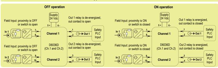
Description: For this application, enable input line fault (open or short) detection and direct input to output transfer function, by set the internal dip-switches in the following mode (see instruction manual for more information):
