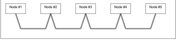
The units are connected to the nodes so that the line appears as a continuous connection starting from the first node and ending at the last node.
