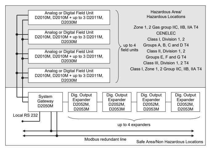
Field units may be Analog or Digital. Each Analog unit accepts up to 3 expanders to increase input capabilities. Up to 4 digital output repeaters can be added to the system in order to reflect the status of digital units in Safe Area/Non Hazardous Locations. Specifications of every module are described in detail in the following sections.
