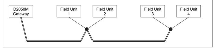
The length of the connections from a node to a unit must not exceed 30 m and the terminating resistor must be activated in the unit at the end of the BUS line (called the trunk) e.g. in unit 4 (see Section 8.4).
