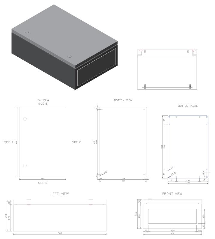
NOTE: gland plate on side D only for carbon steel enclosure, not available for stainless steel enclosure.
