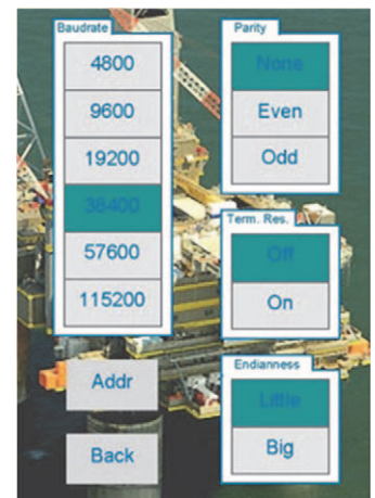
This image is shown when touching the "Modbus" cell in the set up menu screen. Here is possible to set Modbus communication parameters as baudrate, parity, terminal resistance, endianness and address, touching related cells. These parameters are saved in PSO1250 memory and also held after AC1 and AC2 supply shutdown.
