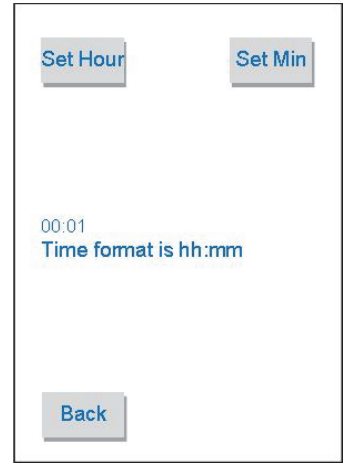
This image is shown when touching the "Set Time" cell in the set up menu screen. Here is possible to set Hour and Minute touching related cells. 24 hours Time format is hour:minute (as hh:mm). Current setting is shown in numeric format. Time is not kept after AC1 and AC2 supply shutdown.
