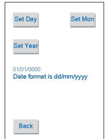
This image is shown when touching the "Set Date" cell in the set up menu screen. Here is possible to set Day, Month and Year touching related cells. Date format is day/month/year (as dd/mm/yyyy). Current setting is shown in numeric format. Date is not kept after AC1 and AC2 supply shutdown.
