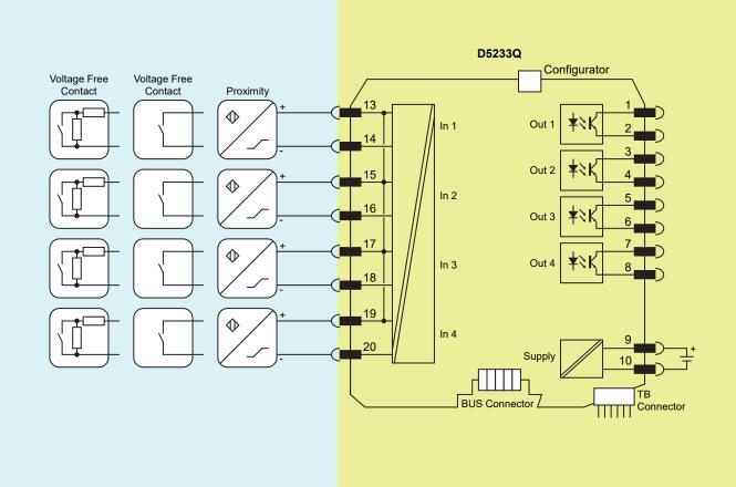
D5233Q used as double channel with Duplicator or Fault Output Configurator
