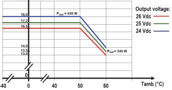
Pout (W) ↑ Valid for AC input voltage nominal range 200 to 240 V<sub>rms</sub> (± 10%)
