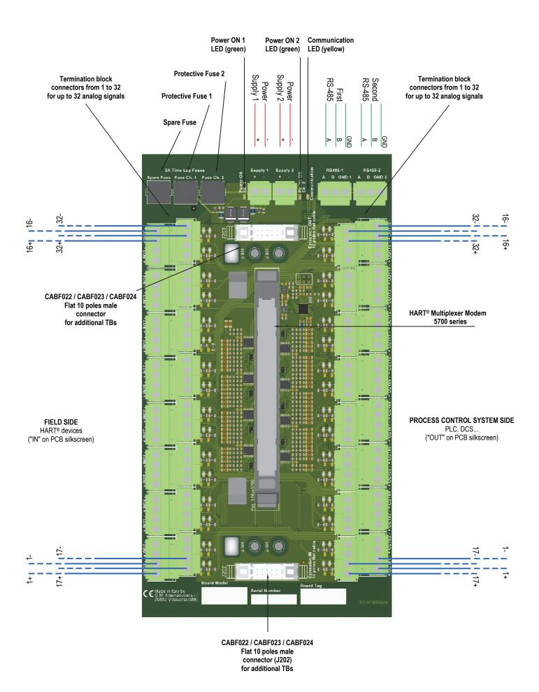
Note: Do not swap field HART® devices (indicated by "IN" on PCB silkscreen) and process control system PLC, DCS... (indicated by "OUT" on PCB silkscreen) connections.
