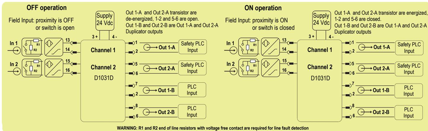
**Description:** For this application, enable input line fault (open or short) detection and direct input to output transfer function, by set the internal dip-switches in the following mode (see page 13 for more information):
