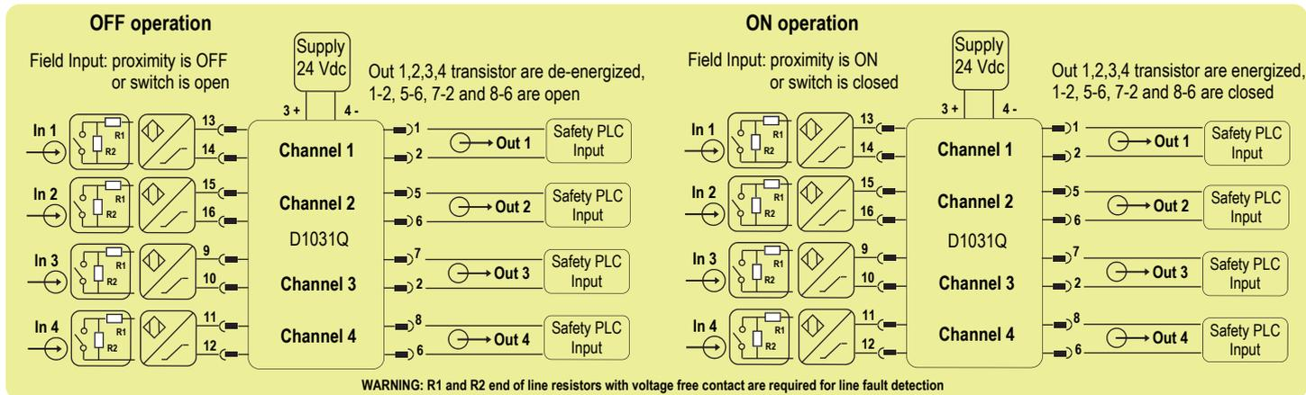
**Description:** For this application, enable input line fault (open or short) detection and direct input to output transfer function, by set the internal dip-switches in the following mode (see page 11 for more information):
