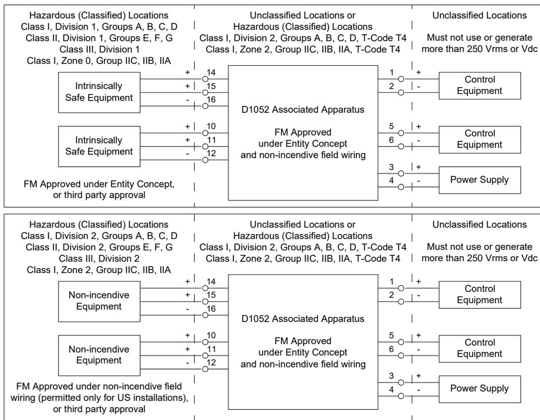
Non-incendive field wiring is not recognized by the Canadian Electrical Code, installation is permitted in the US only.
