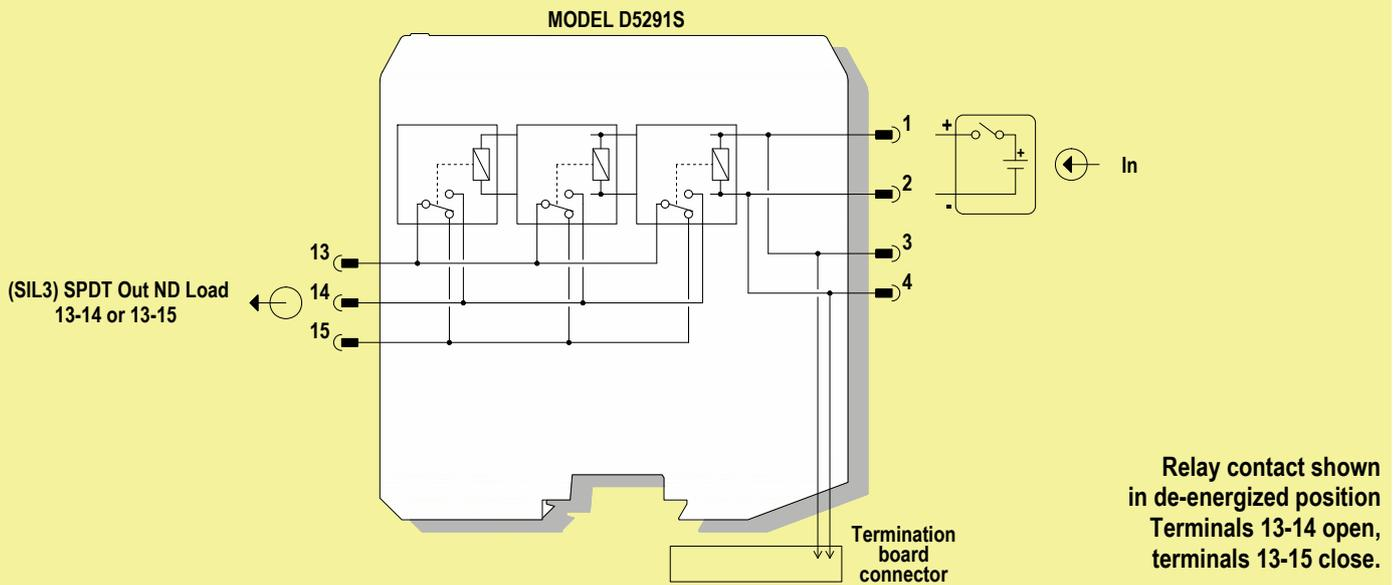
**SIL3 Safety Function for ND load (energized in fail safe state) is available at terminal blocks 13-14;
