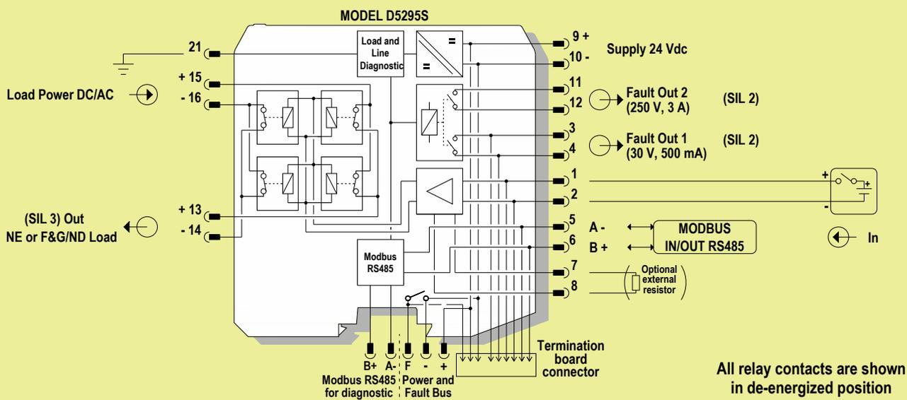
To prevent relay contacts from damaging, connect an external protection (fuse or similar), chosen according to the relay breaking capacity diagram.
