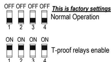
**WARNING:** after T-proof test, dip-switch 1-2-3-4 **must be set** to "OFF" position for normal operation.
